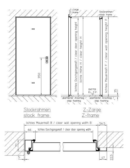
We manufacture to your specifications. Clear wall opening (F) = distance between bottom edge of lintel and top edge of unfinished floor Clear height (H) = distance between bottom edge of lintel and top edge of finished floor
