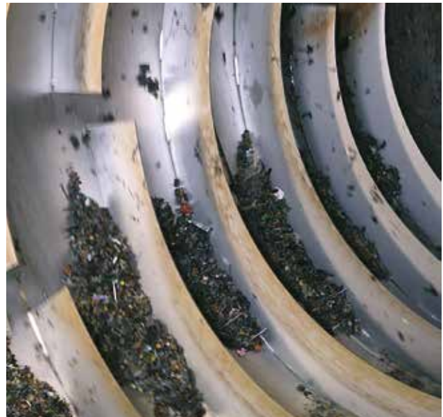
50 l screenings removed per rotation.
