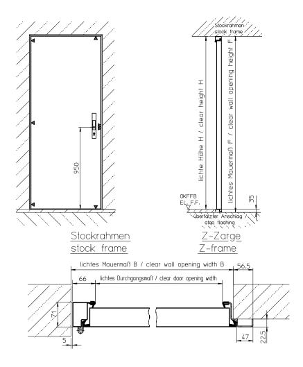
We manufacture to your specifications. Clear wall opening (F) = distance between bottom edge of lintel and top edge of unfinished floor Clear height (H) = distance between bottom edge of lintel and top edge of finished floor
