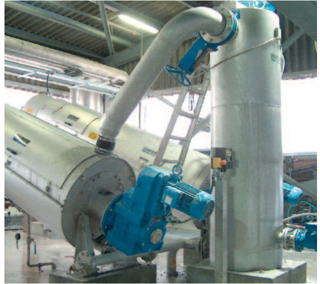
Paper factory SCA Oftringen (CH) HUBER ROTAMAT® Screw Press RoS 3
